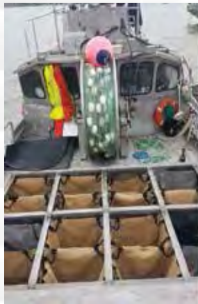
Matthew Kobel of Naknek used Vessel Upgrade Grant funds to flush deck and modify fish holds on his bowpicker in preparation for installing a new RSW unit.
