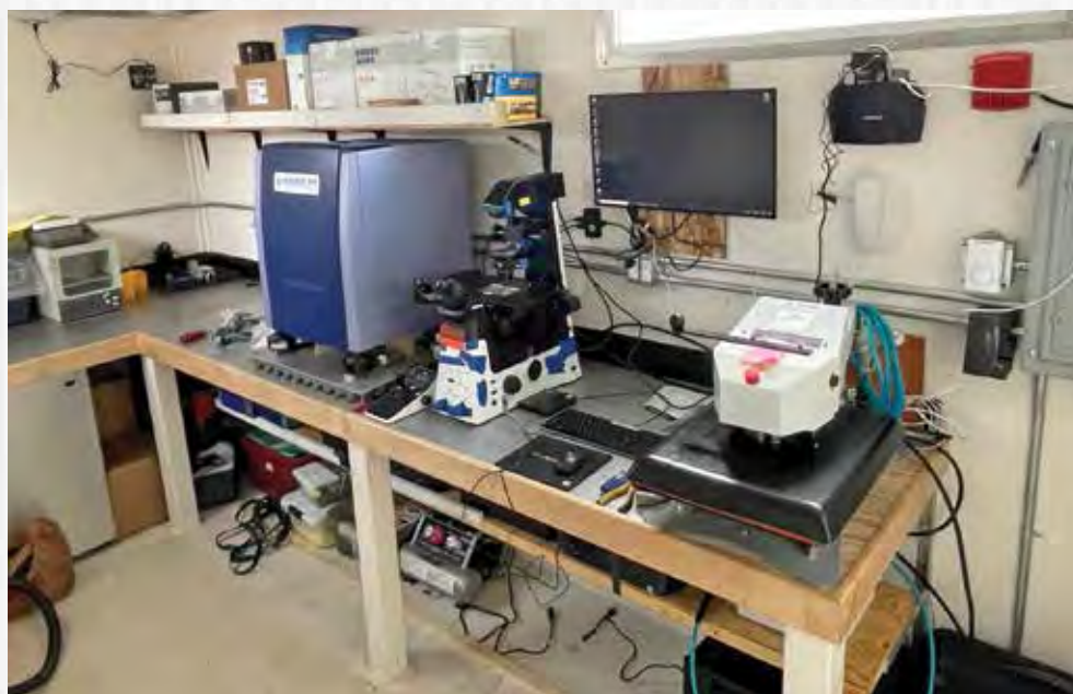
The at-sea genetics and scale lab showing the Fluidigm EP1 (center, tall, blue), The Nikon microscope (just left of the computer screen), and the Knight heat press (right, end of the bench).
